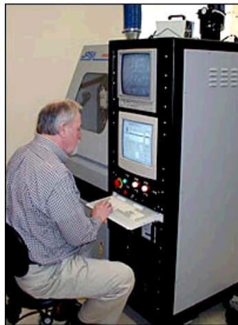
Lamar Bullock, photonic laboratory manager, operates the ATMC's new IX-300 excimer UV laser micromachining system.
